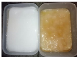
Figure 2. synthesis of bacterial cellulose with the addition of Ammonium Sulfate (left) and yeast extract (right) [16].
